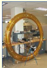
Torus: 1.8 m ring diameter, 0.15 m tube diameter, and 46 \mu m thick (aspect ratio = 0.08)
