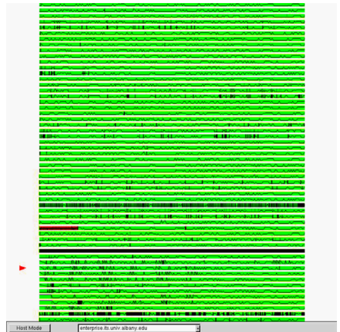
Fig. 5. Summary display showing per host activity. Remote hosts are shown here. Variations from one host to another are observable, as well as variations within single hosts.
