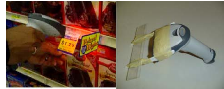
Figure 2: L-Shopper scanning barcode, R-Modified barcode reader
