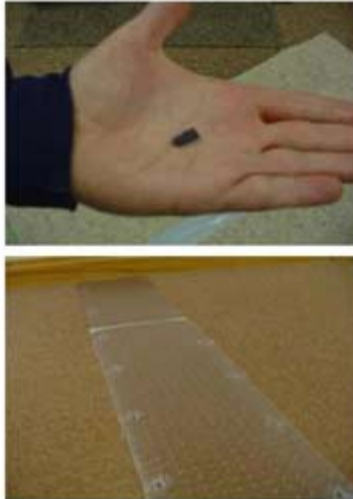
Figure 2: An RFID Tag and a Carpet Strip with Embedded Tags.
