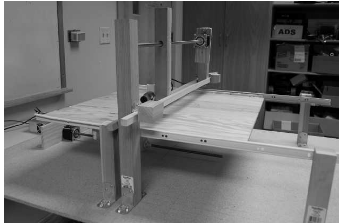
Fig. 4. Model of the Cartesian Robot.
